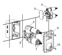
Remove the protection(5) on the valve kit(4). **NOTE**: Don't drop the O-rings(6), don't turn the cartridge spline(7) when install it. The holes on the bottom of the valve kit should be aligned with the holes in the mounting box. Install the valve kit into the mounting box kit, tighten the screws(8).
